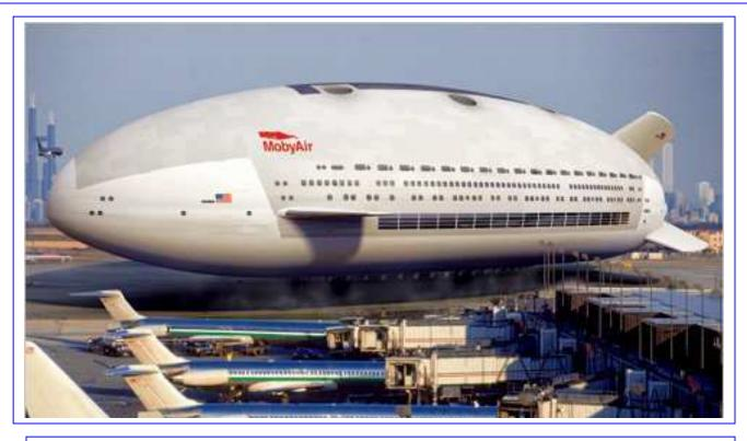
Even though the Aeroscraft dwarfs the largest commercial airliners, it requires less net space on the ground than any plane because it doesn't need a runway. The airship takes off and lands like a helicopter: straight up and down.
